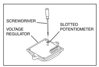
Figure 15. Voltage Adjustment Potentiometer
